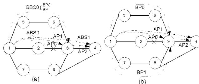
Fig. 3. Recovery schemes using WBS.
