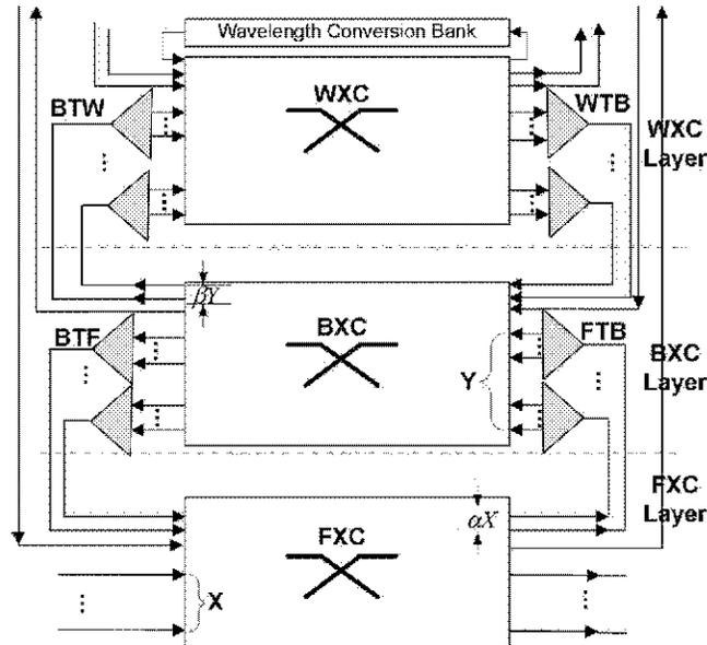
Fig. 1. Reconfigurable multilayer MG-OXC.
