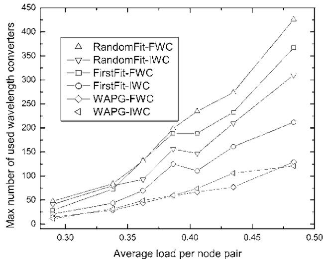
Fig. 7. Maximum number of used wavelength converters ( $\beta=1$ ).
