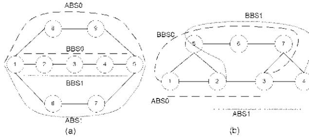
Fig. 4. Backup bandwidth sharing using WBS.
