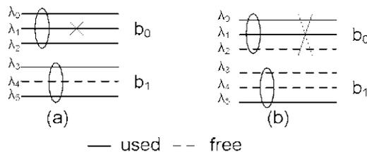
Fig. 5. Band swapping and merging for intralink failure restoration.
