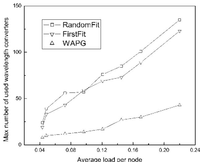
Fig. 11. Maximum number of used wavelength converters ( $\beta=0.75$ ).
