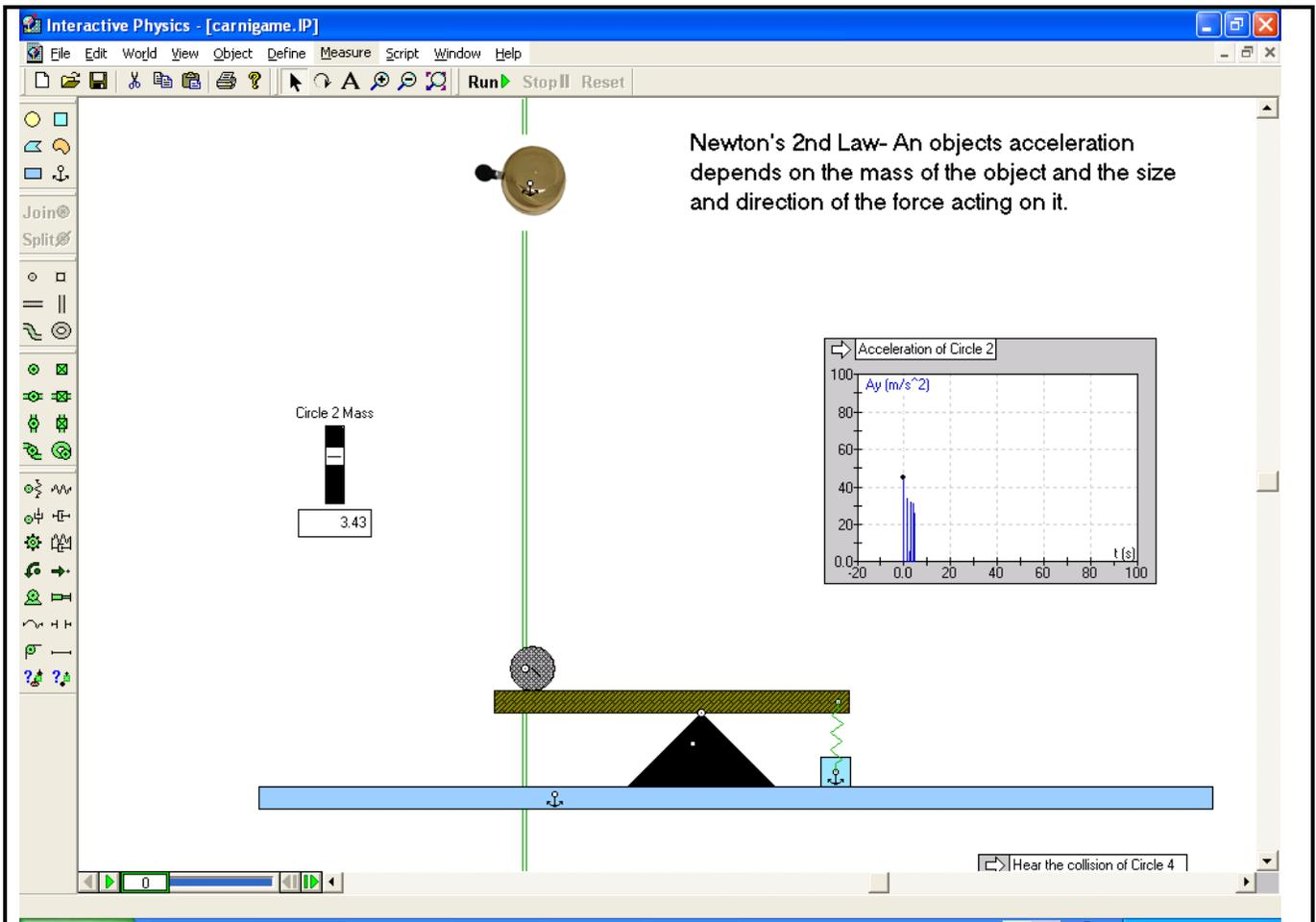
In this model the spring attached to the board is constant. The mass on the grey ball is all that can change. If the same force is applied and the ball is heavier the acceleration will be less and the ball will not be able to travel upwards to hit the bell.
