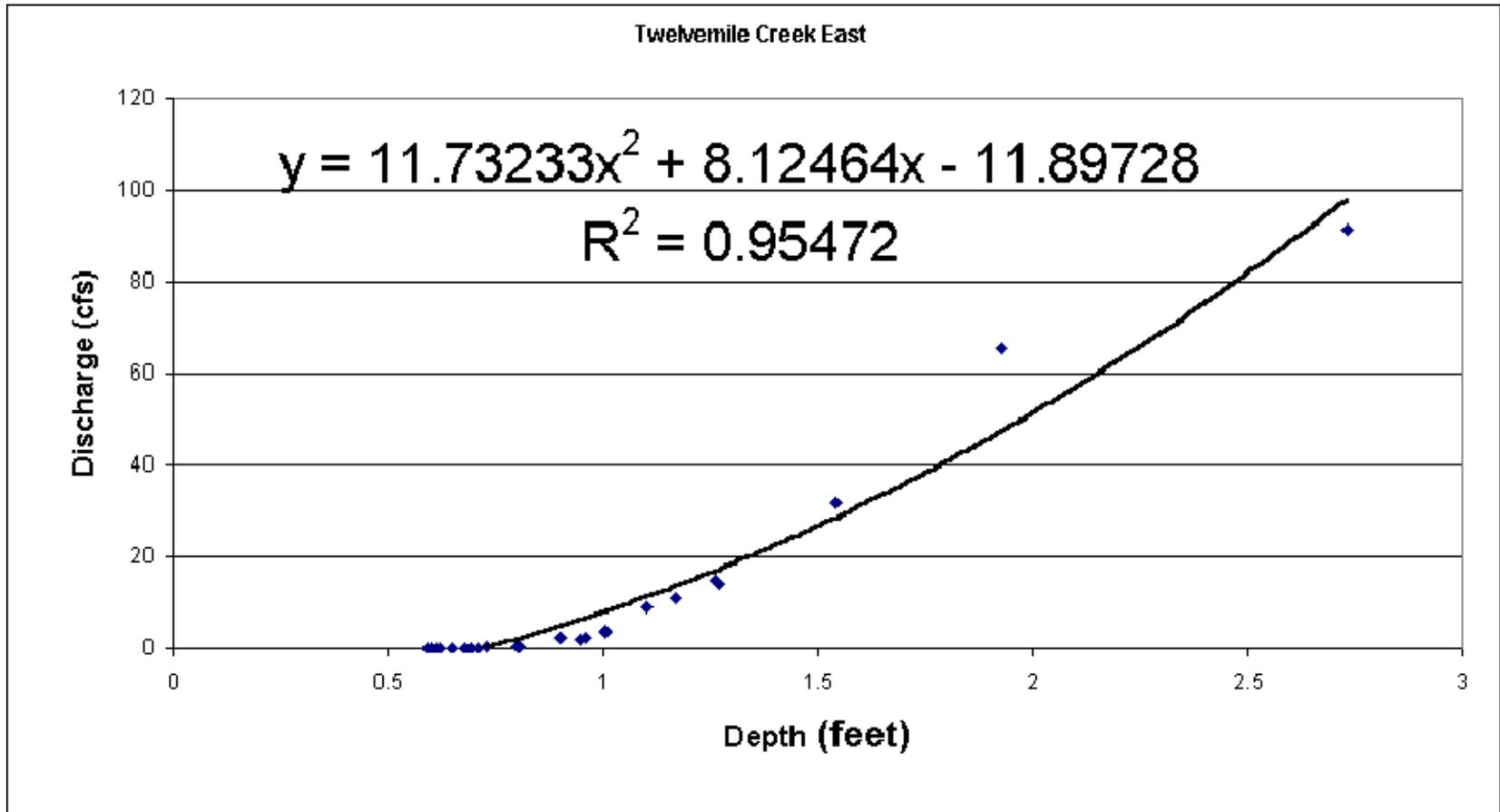
Figure 3. Rating curve for Twelvemile Creek East to be used for creek depths 2 feet or higher.
