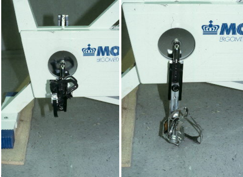
Figure 2: Adjustable pedal shaft mechanism and cranks
