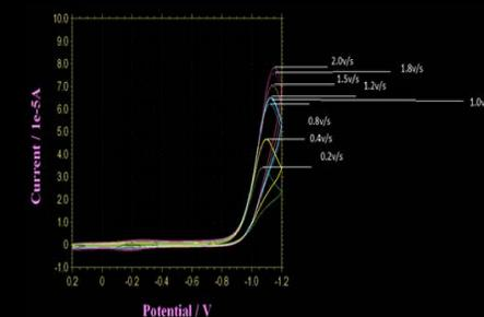
1.3 mm nitromethane in 0.1M acetate buffer at different scan rates.
