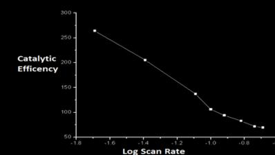
1.3Millimolar nitromethane at different Scan rates
