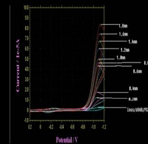
inosoxy/DDAB/PG peaks at different concentrations of nitromethane in 0.1 M acetate buffer at 0.1 V/S scan rate.
