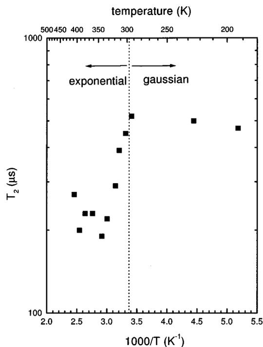
FIG. 3.  $T_2$  measurements on the NIST sample. The measured  $T_2$  represents the decay of the spin-echo envelope and thus is an average over the sites. Above 300 K,  $T_2$  is shorter and describes an exponential decay. This suggests that motion-driven fluctuations in the quadrupole interaction control  $T_2$  above 300 K.
