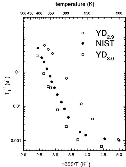
FIG. 5. Relaxation rate  $T_1^{-1}$  for all three samples at 8.4 T. There are two temperature regimes, as seen most distinctly for the NIST sample. Below 250 K,  $T_1^{-1}$  is more or less independent of temperature. Above 300 K,  $T_1^{-1}$  increases according to a thermally activated process. Note that the rates  $T_1^{-1}$  increase markedly in the high-temperature region as the sample is made increasingly sub-stoichiometric.
