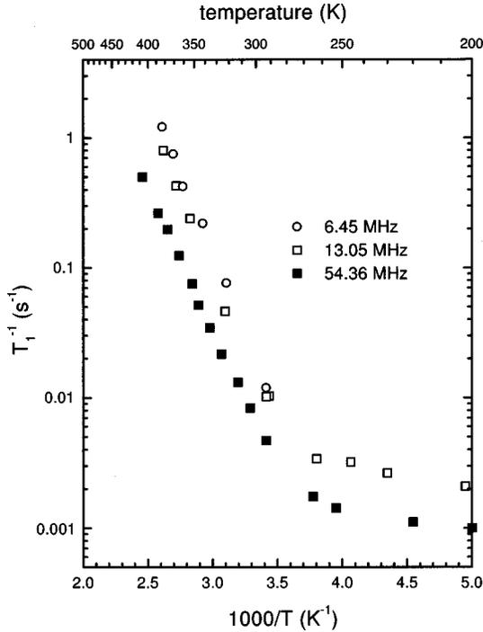
FIG. 6. Relaxation rate  $T_1^{-1}$  at three frequencies in the NIST sample. A weak frequency dependence ( $\approx \omega^{-0.7}$ ) is apparent in both temperature regimes. Note the wide range of measurement frequencies.
