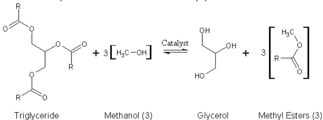
There are two waste products that come from this biodiesel production. The main by-product of the trans-esterification process is glycerin. The second waste stream is from the final biodiesel wash cycle which removes residual methanol, glycerin, and acid salts. After residual oil removal the wash cycle water is safe to dispose of down the drain.
